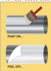
on construction site to provide mechanical protection against nicks, abrasion, scratches, and over-spray to the surfaces that it covers. MCI Peel-off Coating can be used to protect non-porous surfaces such as walls, ceilings, floors, windows and light fixtures: one coating to do it all. In addi-
